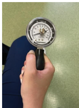
Figure 1: Hand-held dynamometer (private archive)
